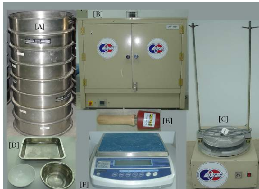
Fig. 7-12: Sieve Analysis Apparatus: (A) Sieve aperture sizes, (B) Dry oven, (C) Sieve shaker, (D) Mortar & Tray, (E) Rubber pestle, (F) Balance
